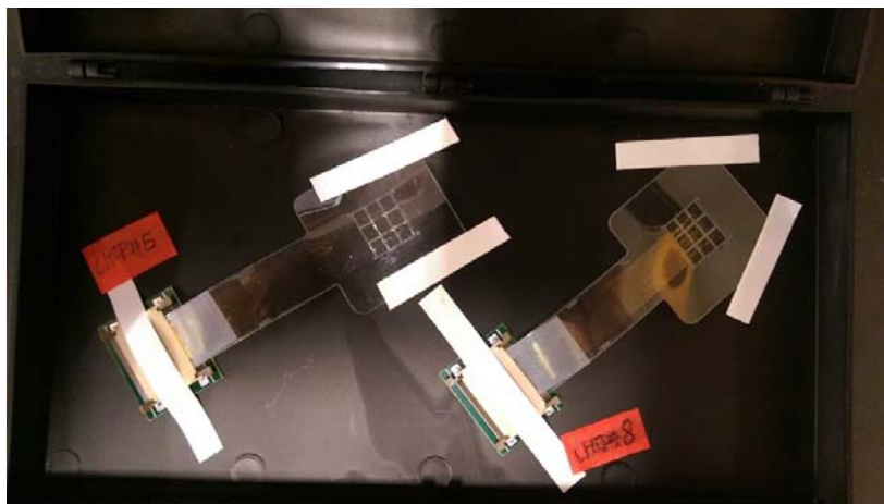
Figure 8. Copper tape-secured SiNW nanoFET meshes after assembly in an anti-static container before shipping.
