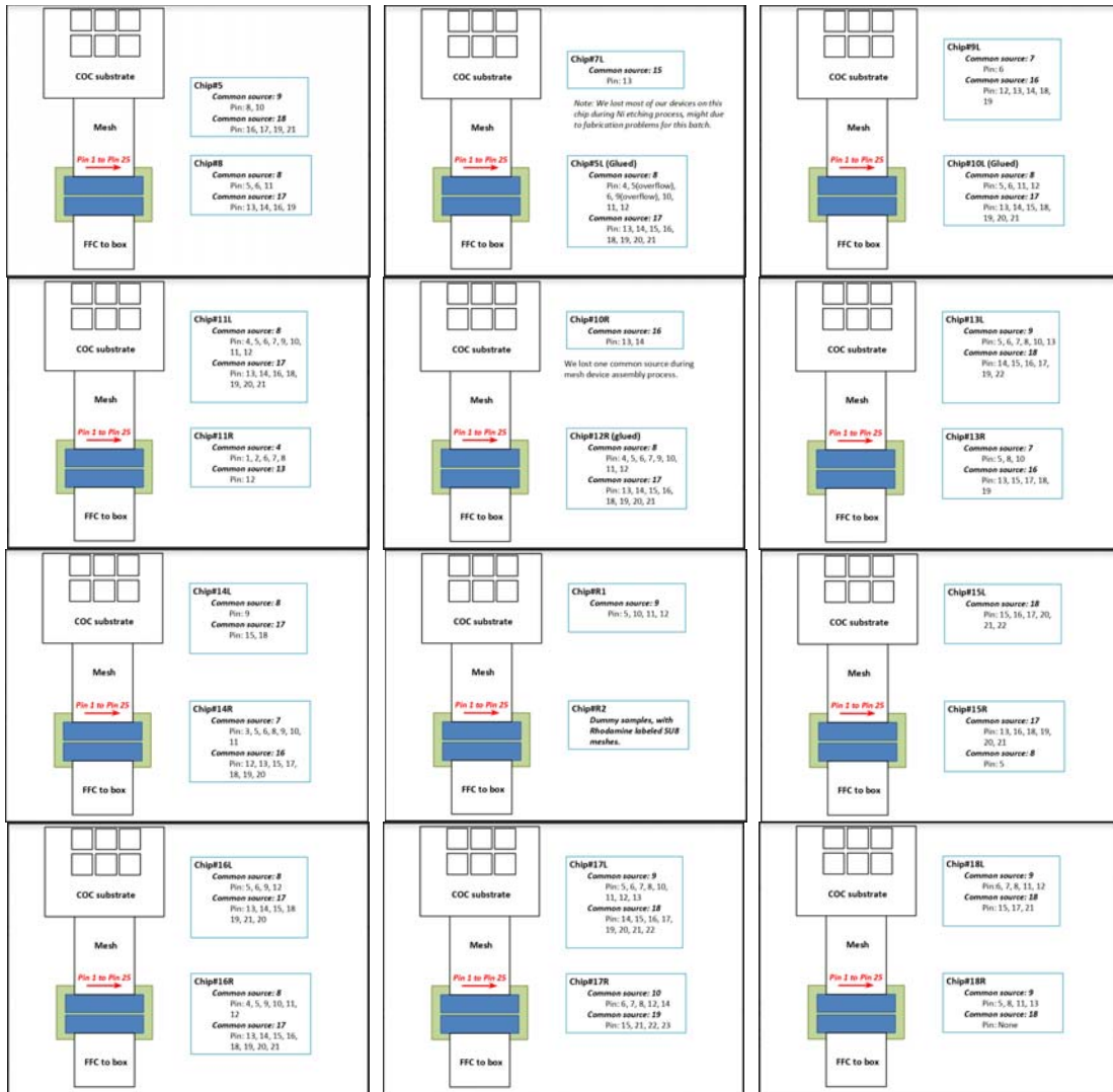
Figure 7. Detailed pin assignments for each SiNW nanoFET mesh device.
