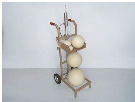
Fig. 2. Bonner Sphere Spectrometer detection system.
