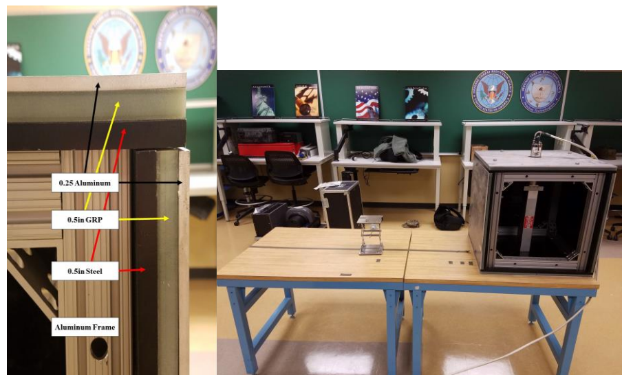
Fig. 1. The picture on the left shows the surrogate vehicle with layered materials (from outer to inner): 0.25in Aluminum, 0.5in GRP, and finally 0.5in steel. The picture shows the materials without the other shielded sides of the surrogate vehicle. The picture on the right depicts the experiment with a radioisotope placed a set distance from the surrogate vehicle.
