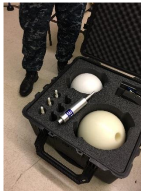
Fig. 2. Bonner Sphere Polyethylene Spheres and \text{LiI}(\text{Eu}) Detector.
