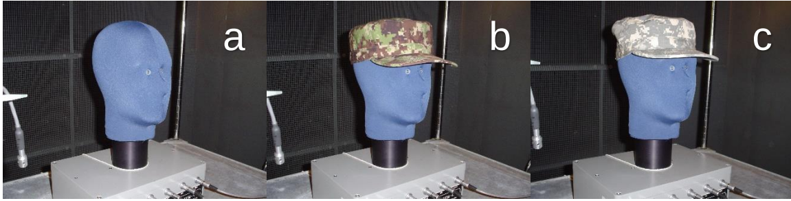
Figure 1. Sweating thermal manikin head (a), prototype Afghanistan military cover (b) and US Army current issue patrol cover (c)
