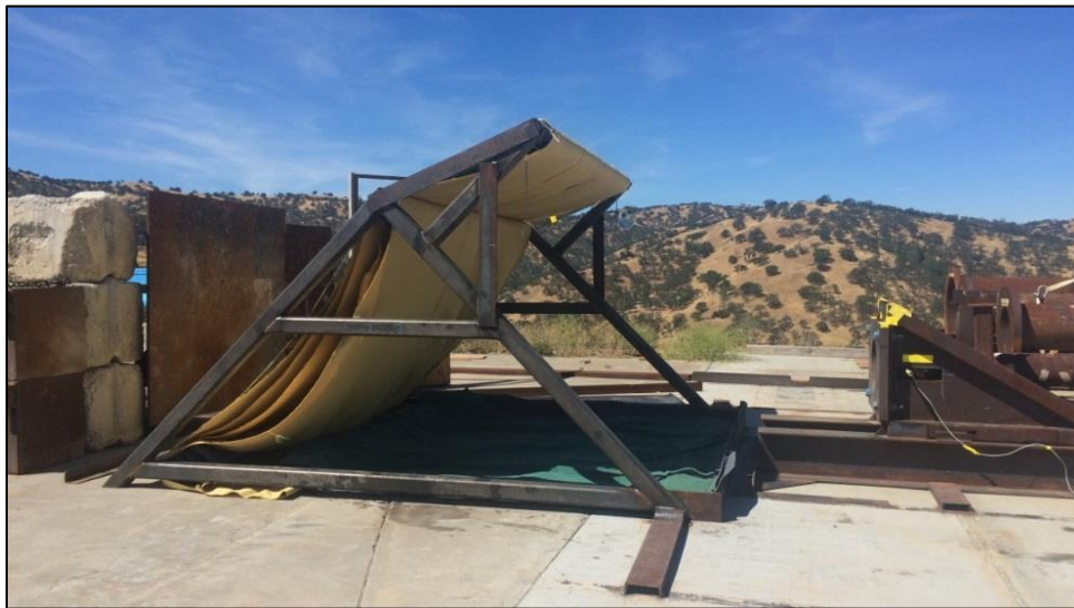
Figure 12. Photograph of the high-pressure shock tube and the new soft-capture fragment collection system used in Tests 29 to 39 conducted in June 2015.
