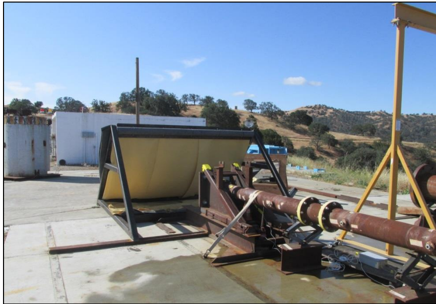
Figure 5. Photograph of the high-pressure shock tube and the original soft-capture fragment collection system used in Tests 22 to 25 conducted in May 2015.
