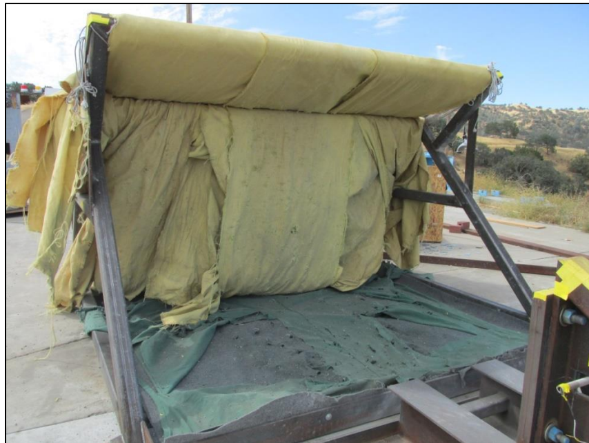
Figure 14. Post-test picture of new soft-capture fragment collection system after high-pressure test (Test 36).
