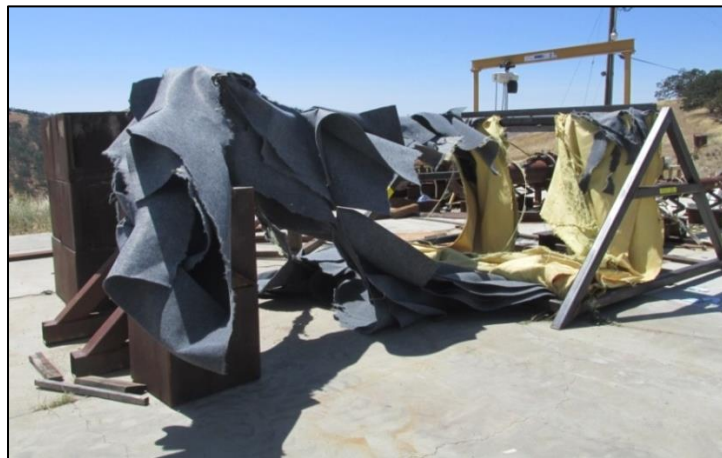
Figure 7. Photograph of damage to the original soft-capture collection system following Test 25.
