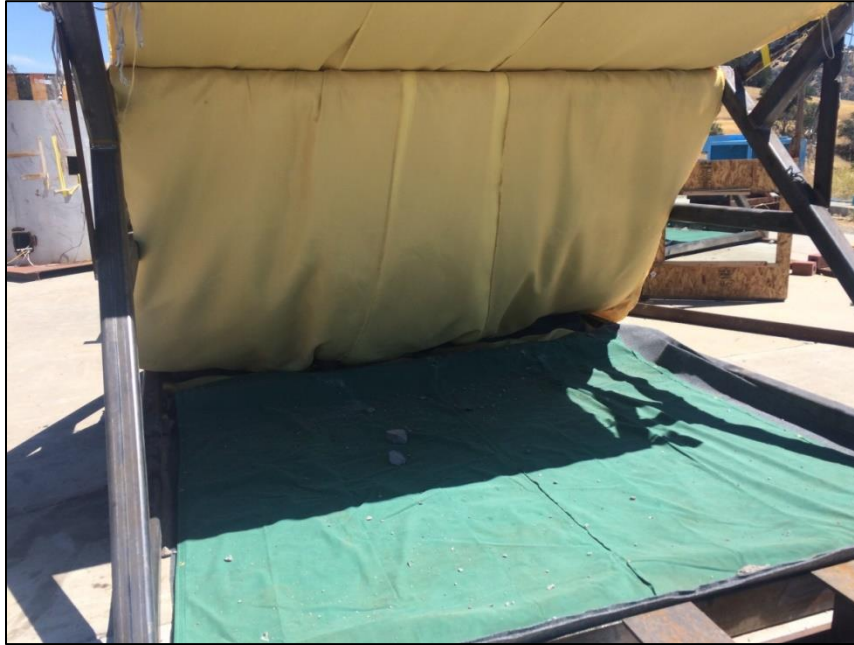
Figure 13. Post-test picture of the new soft-capture fragment collection system after a low-pressure test (Test 29)
