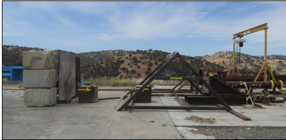
Figure 8. Photograph of the high-pressure shock tube and pressure gages mounted on concrete-filled steel blocks used in Test 26, 27, and 28.
