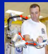
Adjustable Arm Geometry (3 passive links)
