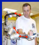
scapula joint for shoulder elevation
