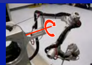
Shoulder Elevation (Scapula Joint)
