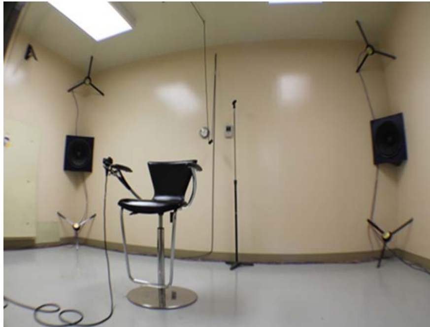
Figure 2: Real-Ear-At-Threshold Test Chamber, Air Force Research Laboratory
