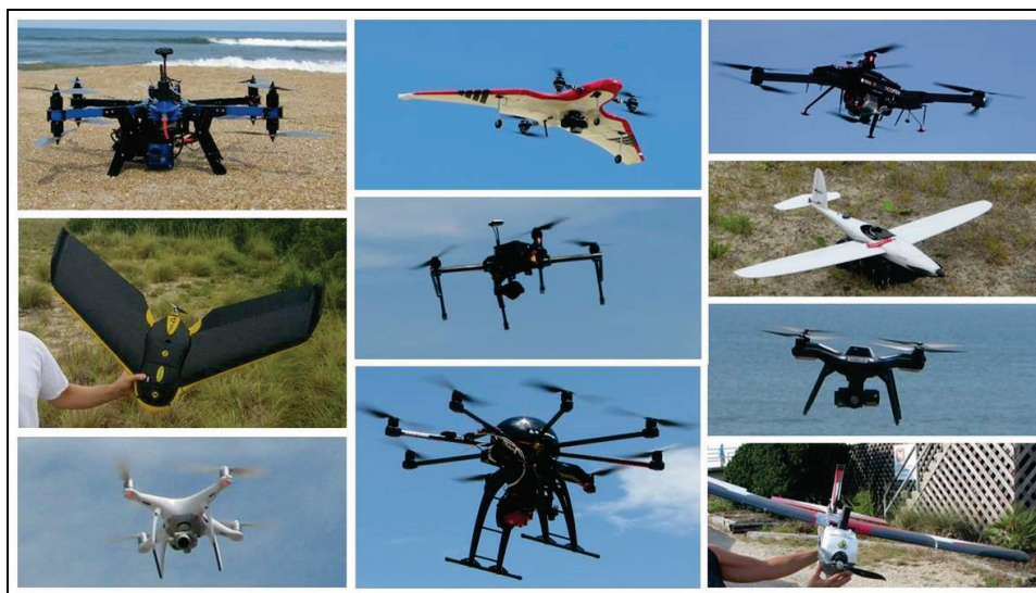
Figure 1-3. Different UAS platforms flown at the June Duck Pilot UAS for FRM Field Experiment. By column, left to right (3DR X8+, SenseFly eBee, DJI Phantom 4 Pro, BirdsEyeView FireFLY6 Pro, DJI Matrice 100, Multirotor G4 Skycrane, Riegl RiCopter, Sky-watch Cumulus, 3DR Solo, PrecisionHawk Lancaster.
