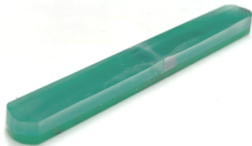
Epoxy-A/PCB cured sample
