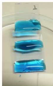
Fig.4 Tilted S-layer patterned glass slide demonstrating the water-retention capability of the S-layer coating. For better visualization water was stained with methylene blue.
