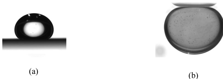
Fig.6 Contact angles of a high- and a low-density fluid on/under a wtSbpA S-layer coated glass slide in water. (a) Diiodomethane (contact angle = 140°) and (b) Olive oil (contact angle = 155°).
