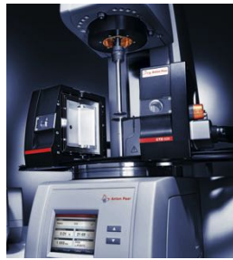
Fig.29 Rheometer MCR 702 (Anton Paar) shown with 2 discs and open temperature control jacket. Torque resolution is 0.1\text{ nN} \cdot \text{m}
