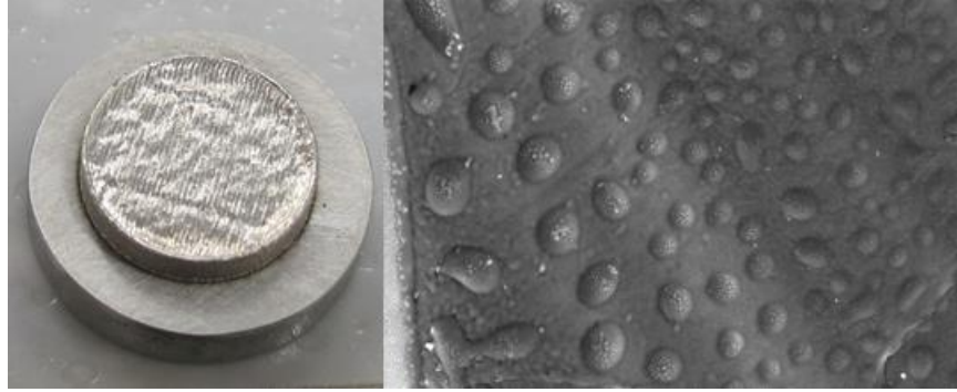
Figure 13: A corrosion test sample made from Ce-doped material.
