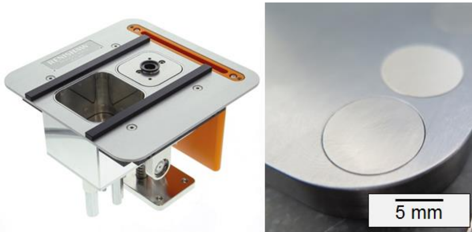
Figure 11: Minimizing required powder volumes using a modified reduced build volume
