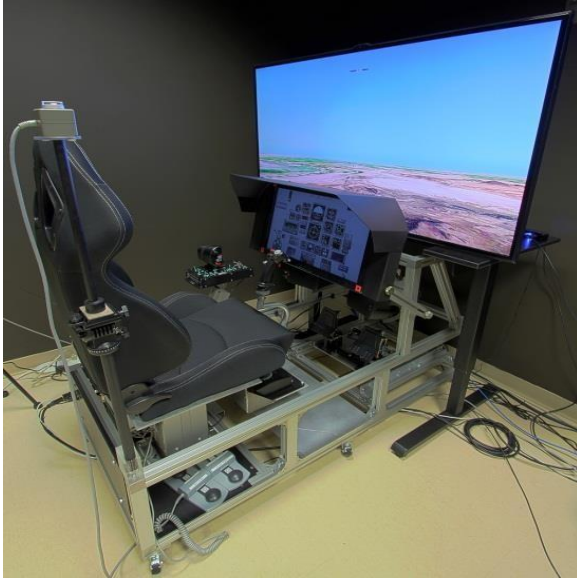
Figure 1. NAMRU-D fixed-base flight simulator cockpit
