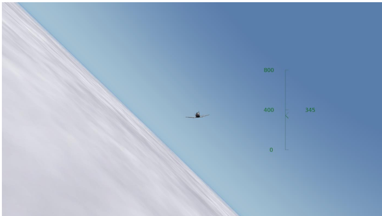
Figure 3. Screen shot of the Variable Following-Distance Task (VFDT), with 400 feet as the requested following distance, and 345 feet as the actual distance.
