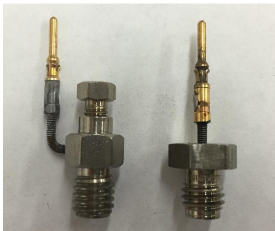
Figure 6. Modified Valco external/internal reducing union (left) and Swagelok cap (right) used to make vacuum tight seals and provide easy electrical contact of the temperature probe drift rings to the resistor chain via the gold pin connectors soldered to the short posts drilled into the parts.
