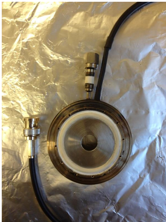
Figure 4. Front view of the drift gas showerhead assembly showing the Faraday plate and insulating ceramic cemented in the center, and the drift gas isolator (left) and BNC signal lead (right) on top of the showerhead base. The electrode post screwed into and supplying voltage to the base is in line behind the BNC signal lead.
