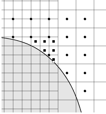
FIGURE 4. Modified least-squares stencil at a coarse/fine mesh boundary. Showing the fine grid Lagrangian interface point (open circle), under-filled fine level least-squares stencil (closed square), and coarse level least-squares stencil (closed circle). In practice, a 5x5 or 7x7 stencil is used so that (4.9) is not rank deficient.
