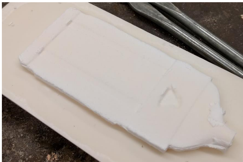
Figure 16. Sintered sample formed via injection molding of a suspension with 51 vol.% \text{Al}_2\text{O}_3 with 5 vol.% PVP.
