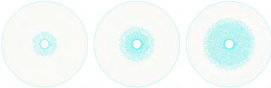
Figure 23: Fracture of brittle disk under core expansion.
