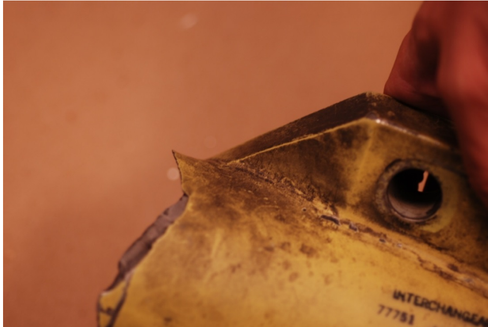
Figure 24. Failed thrust fitting.
