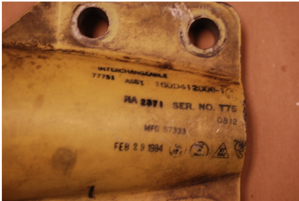
Figure 25. Markings on failed thrust fitting.
