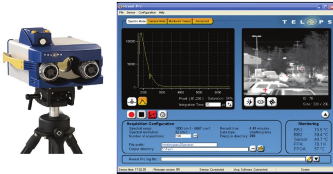
Figure 8: Telops IFTS HSI instrument and data collection.[21]
