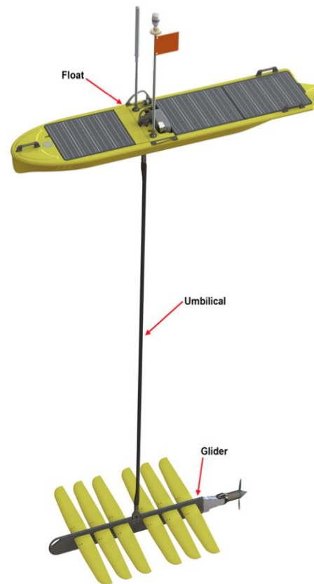
Figure 1 Liquid Robotics SV-3 Wave Glider components. The umbilical is 4 m long.
