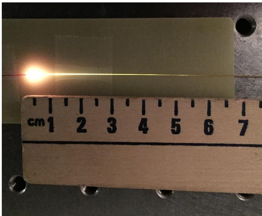
Figure 11. Image of the nanocolloid optical fiber amplifier based on a hollow fiber filled with the nanocolloid of RE phosphor \text{NaYF}_4: \text{Yb}^{3+}, \text{Er}^{3+} in a high-index liquid. The bright trace of visible light is produced by the upconversion emission from the nanocolloid pumped with a 980-nm IR radiation entering the fiber from the left. The pump radiation is delivered via a 980/1550-nm single-mode optical fiber spliced to the hollow fiber using Optical Fiber Splicer System including Fujikura 12S+CT-30 fusion splicer and LFS-004 (SSSOT) splicer/integrity tester.
