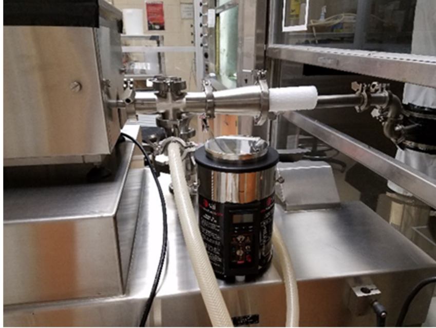
Figure 3. Location of air sampler during milling operations.
