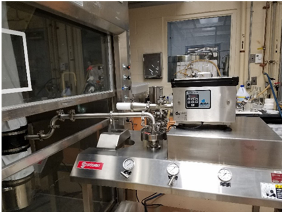
Figure 4. Milling operation setup with approximately 500 g of barcoded Btk spores.
