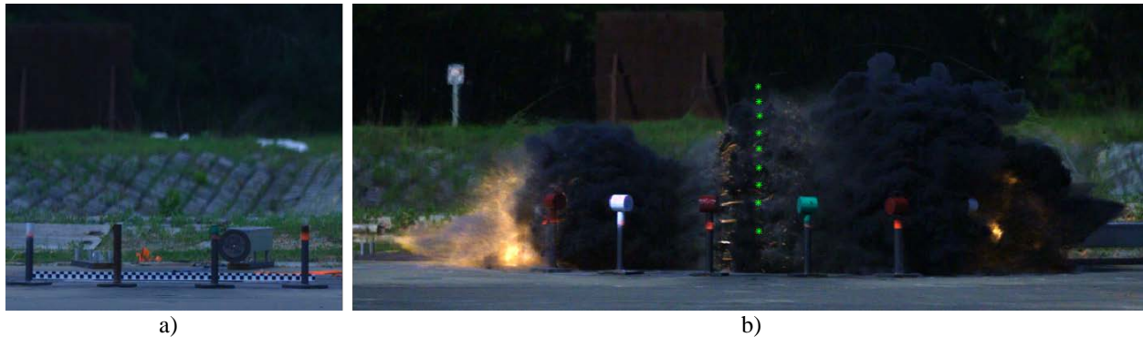
Figure 15. Image analysis examples. a) Each camera used a static image with a checker pattern fiducial to calibrate the image. b) The location of the shock was selected manually for each frame along the centerline and normal to the ground. Previous selections are shown as green markers
