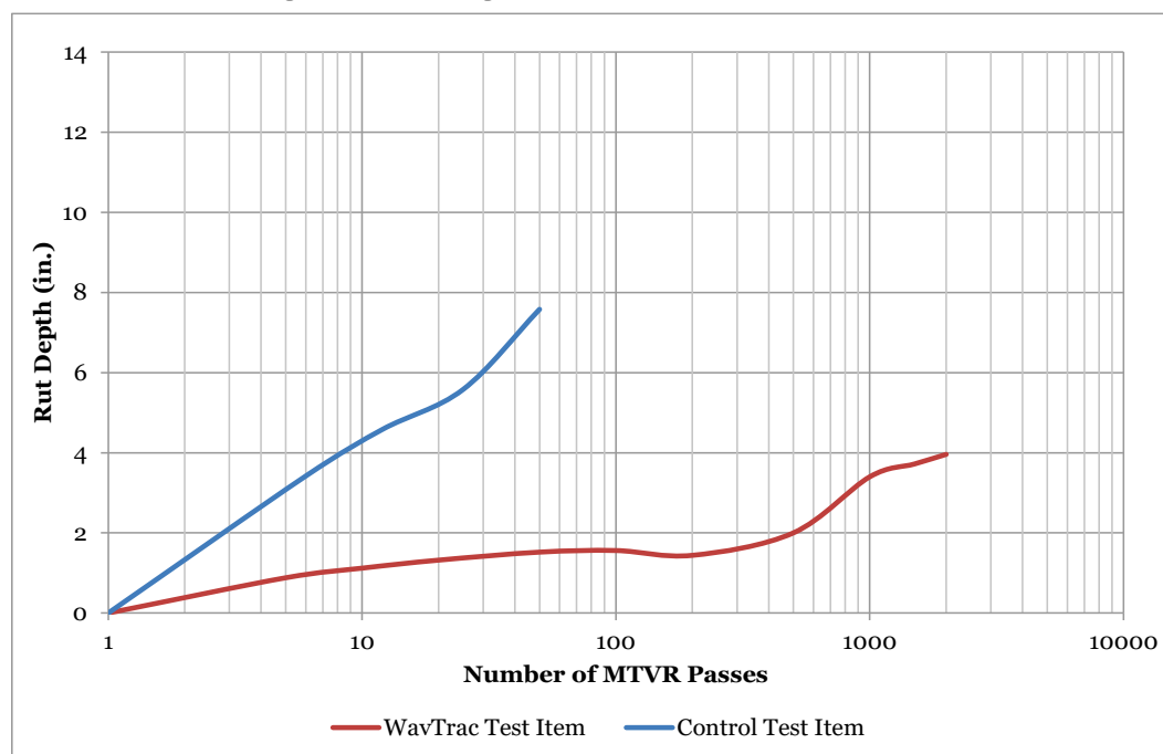
Figure 10. Average rut depth for SP-15 test items.
