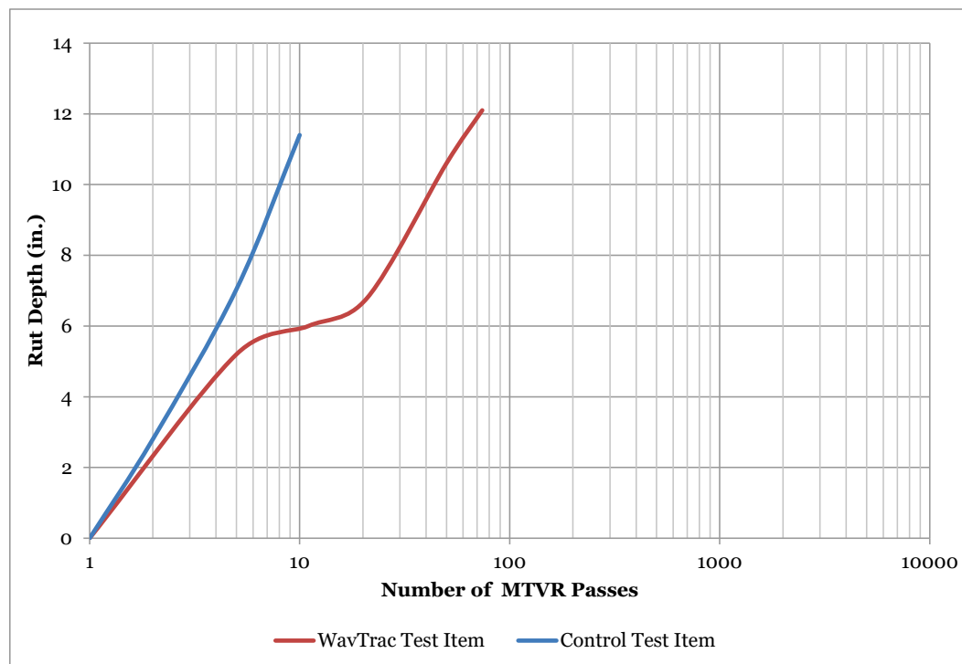
Figure 11. Average rut depth for CL-3 test items.
