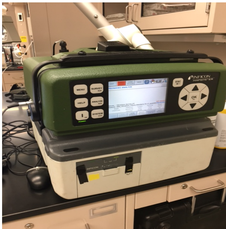
Figure 3.1. The HAPSITE® ER GC/MS Instrument. The HAPSITE® ER analytical module (green) sitting atop a service module.
