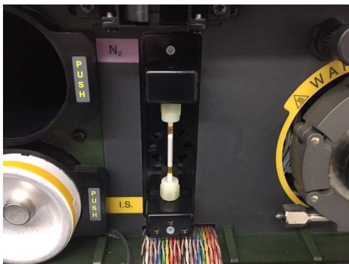
Figure 3.2. Internal concentrator. The concentrator contained three sorbents of varying strengths (Carbotrap Y, Carbotrap C, and Carboxen 1018). After collecting isoflurane from the whole air sample (probe) or from the thermal desorption cycle, the concentrator is heated to rapidly release the collected isoflurane into the analytical column.
