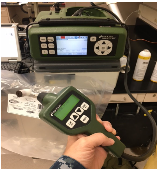
Figure 3.3. Hand-held direct air sampling probe. The probe is drawing sample air from a 5-L Tedlar® bag.
