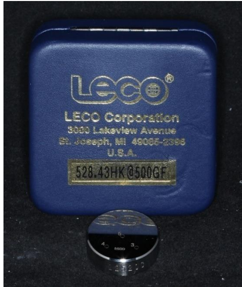
Figure6: Leco 300AT Calibrating Disc
