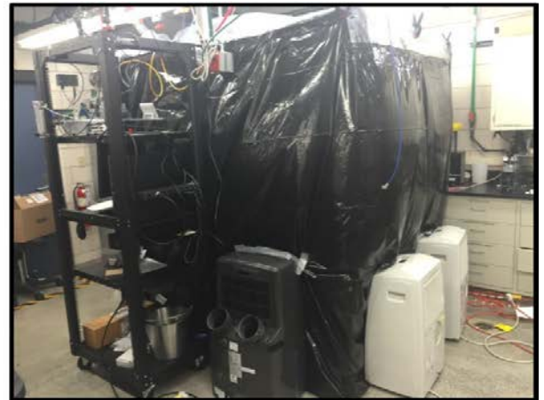
Figure 6. Temperature control using an enclosure (front and back)
