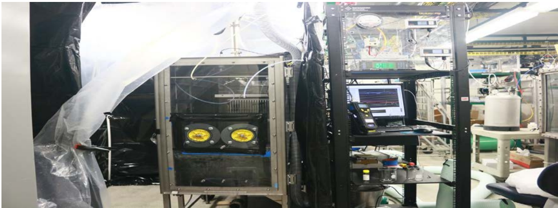
Figure 8. The environmental chamber set-up
