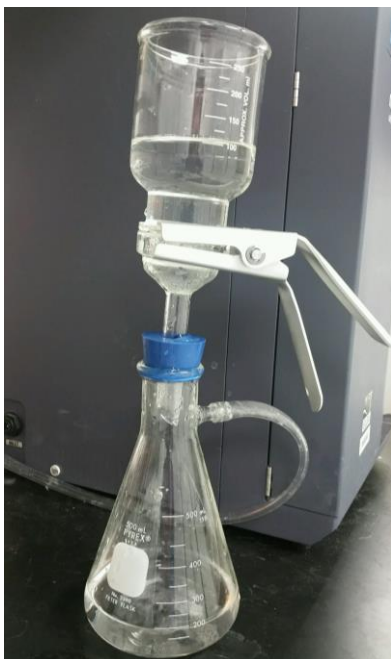
Figure 10. Buchner Funnel Filter Flask Apparatus
