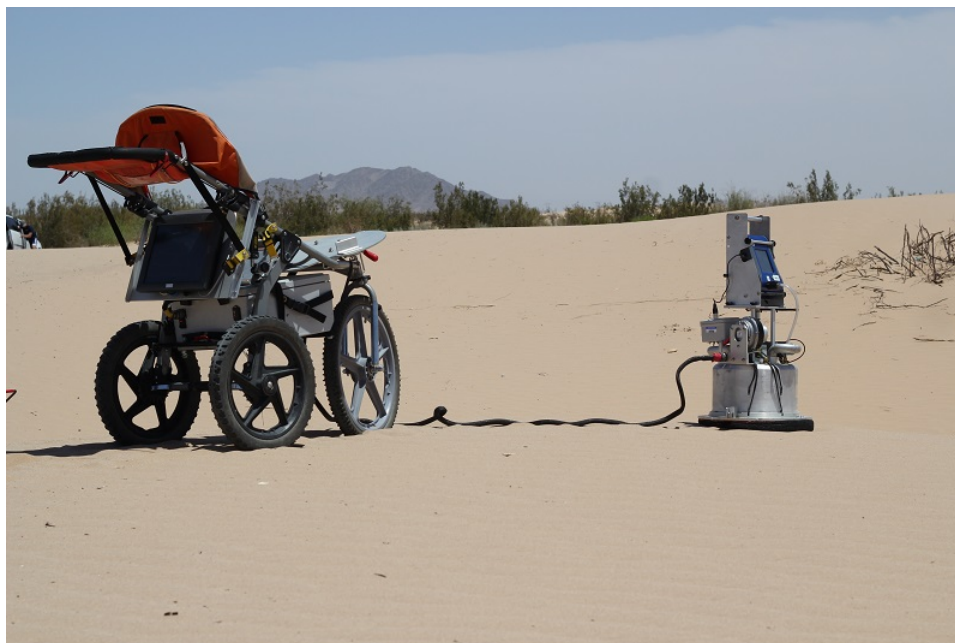
Figure 8. PI-SWERL set up for measurements at site SWD28. The attached carriage is used for transport and holds the battery and software controls.
