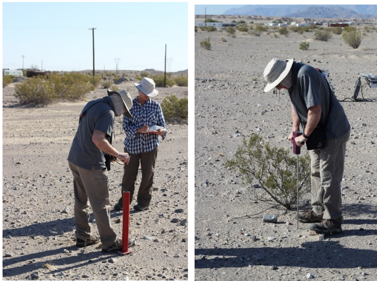
Figure 6. Clegg ( left ) and cone penetrometer ( right ) measurements at site SWD8.
