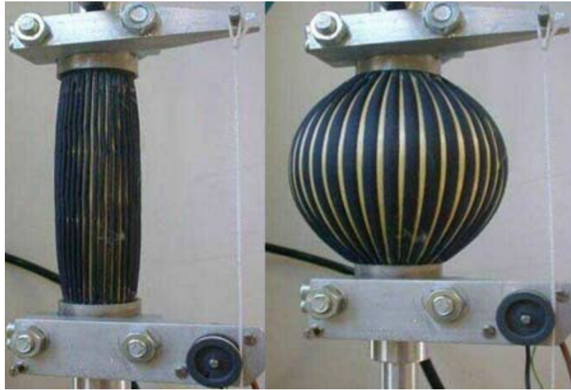
Fig. 12 PPAM in relaxed and contracted states (Reprinted with permission from Verrelst et al. 263 )
