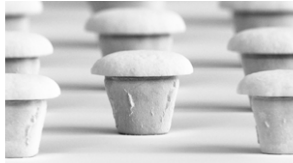
Figure 8. Electroplated electrodes with 10 \mu m wide pillars and rounded tops.
