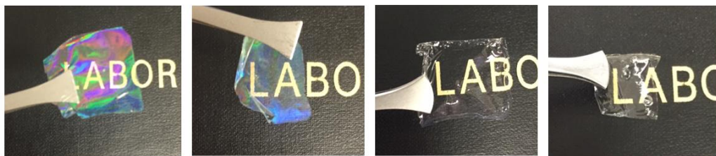
Figure 3. From left to right: macroscopic images of chemically crosslinked P500, stabilized P500, P300, and flat biopolymer film.
