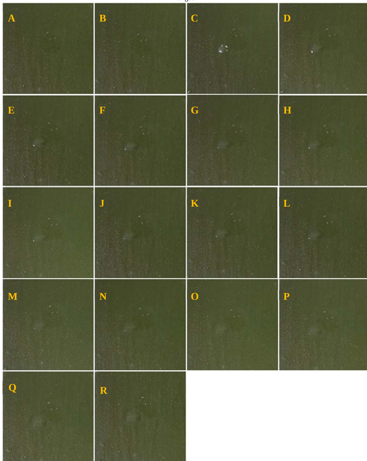
Fig. F2 — MES on Fomblin Y oiled paint. Images of a coupon before application (A) and at 0 (B), 0.5 (C), 1 (D), 1.5 (E), 2 (F), 2.5 (G), 3 (H), 3.5 (I), 4 (J), 4.5 (K), 5 (L), 5.5 (M), 10 (N), 15 (O), 20 (P), 25 (Q), and 30 (R) min following application of the target.
