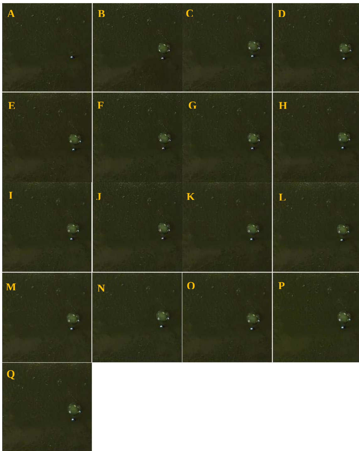
Fig. C3 — DMMP on TH1555. Images of a coupon before application (A) and at 0 (B), 0.5 (C), 1 (D), 1.5 (E), 2 (F), 2.5 (G), 3 (H), 3.5 (I), 4 (J), 4.5 (K), 5 (L), 10 (M), 15 (N), 20 (O), 25 (P), and 30 (Q) min following application of the target.
