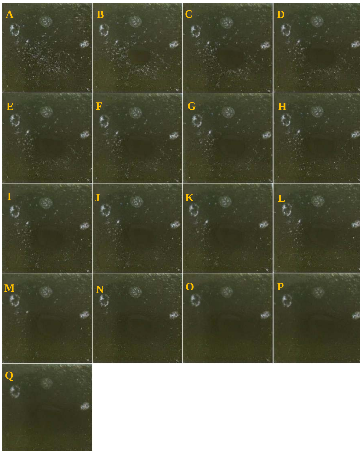
Fig. D1 — DFP on SO1465. Images of a coupon before application (A) and at 0 (B), 0.5 (C), 1.0 (D), 1.5 (E), 2.0 (F), 2.5 (G), 3.0 (H), 3.5 (I), 4.0 (J), 4.5 (K), 5 (L), 10 (M), 15 (N), 20 (O), 25 (P), and 30 (Q) min following application of the target. These images were collected with a glass cover in place to limit evaporation. Reflections from the cover can be seen in some images.
