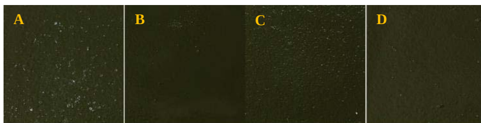
Fig. 3 — Images of painted coupons with hepta-trifluoropropyl trisilanol POSS (A; SO1465) aminopropylisooctyl POSS (B; AM0270); methacrylisooctyl POSS (C; MA0719); and mercaptopropylisooctyl POSS (D; TH1555).
