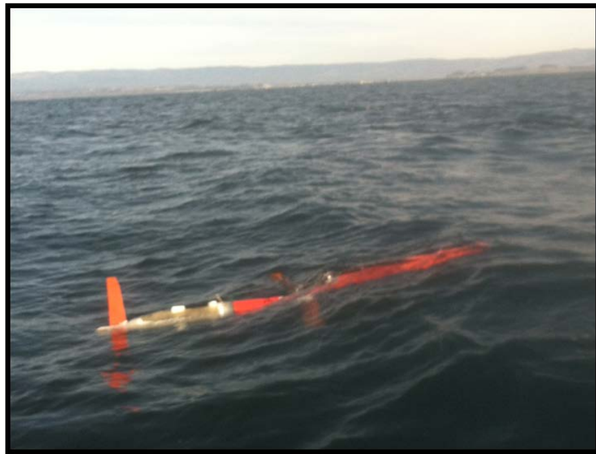
Figure 46. NPS Spray glider with acoustic receiver deployed near Moss Landing on 12-Aug-2014
