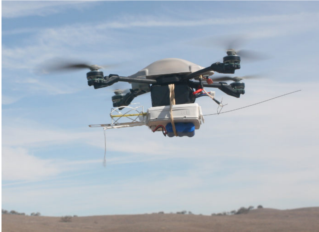
Figure 30. InstantEye MR-VTOL unmanned aircraft with radiosonde attached.
