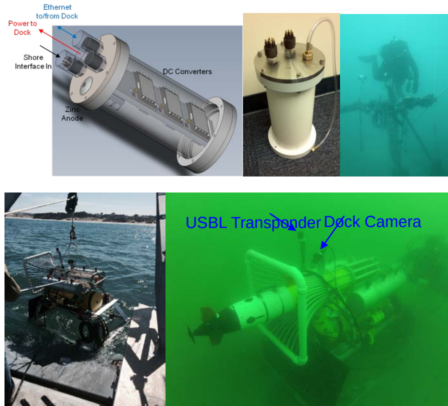
Figure 27: The Electronics Interface between MISO and CAVR equipment, designed, built, and deployed (top), and the REMUS 100 Docking station deployment at MISO and deployed with a docked vehicle (bottom)
