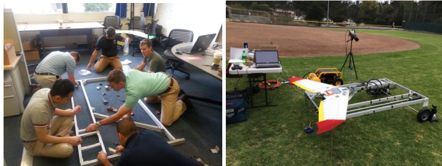
Figure 22: A team of Systems Engineering students design and build a multi-UAV launcher, based on end-user needs and system requirements ( left ) and conduct tests of their prototype design ( right )
