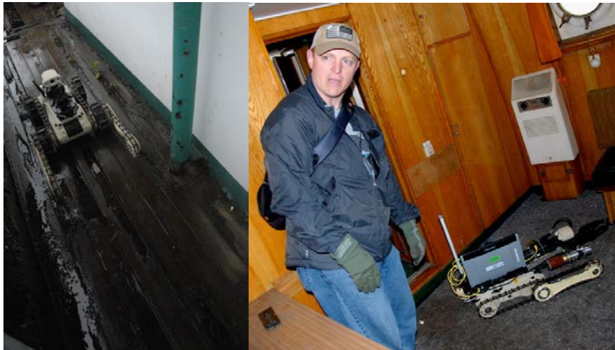
Figure 9. The Micro Tactical Ground Robot (MTGR) is piloted along the hull of the Copernicus target vessel in search for a radioactive substance.
