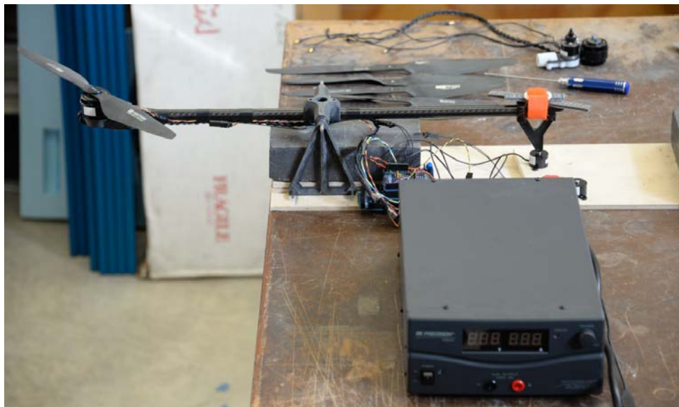
Figure 40: Motor test stand instrumented by summer intern, Kevin-Patxi Le Bras.
