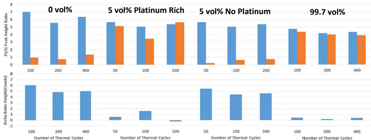
Figure 44: Before Cycling (blue bars, top row) and After Cycling (orange bars, top row) Platinum/Silicon Peak Ratio Comparison for Electrical Bias Effects using 15.5V in 0 vol% Acetic Acid (left column), 5 vol% Acetic Acid Platinum Rich (2 nd from left column), 5 vol% Acetic Acid no Platinum (2 nd from right column) and 99.7 vol% Acetic Acid (right column) which was Calculated from Figure 42 and Figure 43. Bottom Row Shows Delta Value between Before and After.
