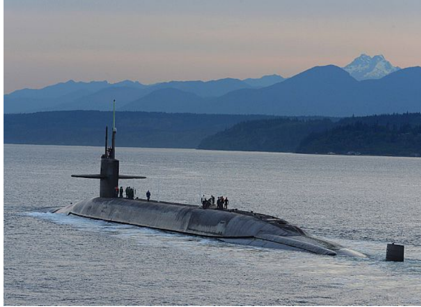
Ohio class submarine at sea. The Ohio class is the current ballistic missile submarine used for strategic deterrence in the U.S. Navy.
