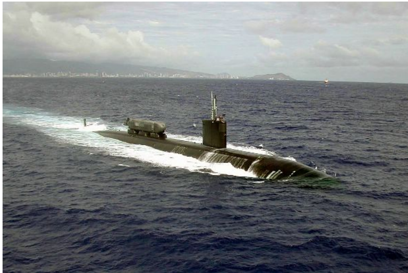
Los Angeles class submarine at sea equipped with the Advanced Seal Delivery System for Special Forces.
