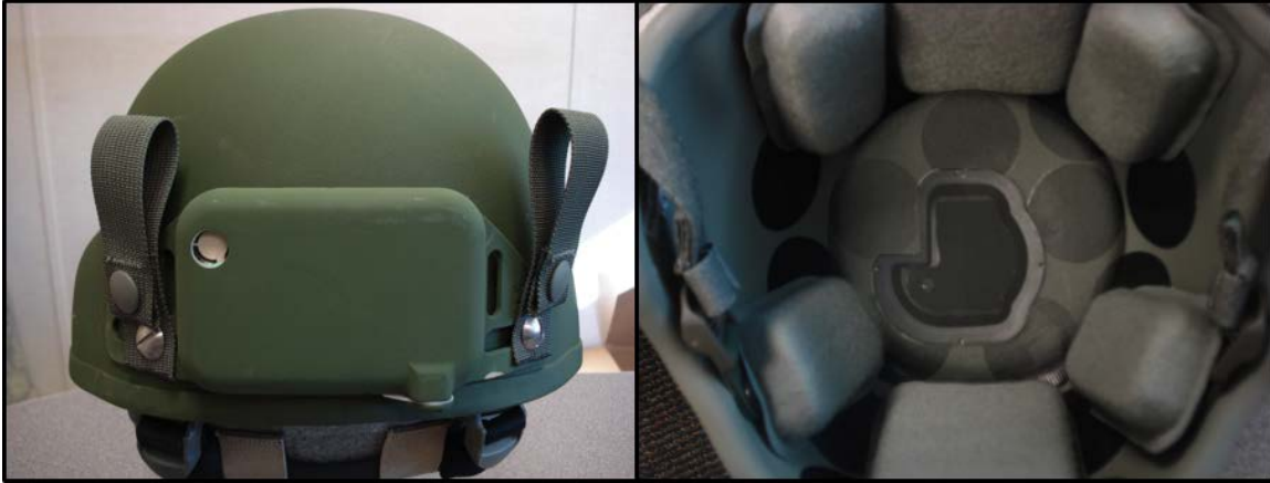
Figure 6. Gen I Helmet Mounted Sensor System (HMSS), externally mounted (left), internally mounted (right). Source: PEO Soldier (2009a; 2009b).
