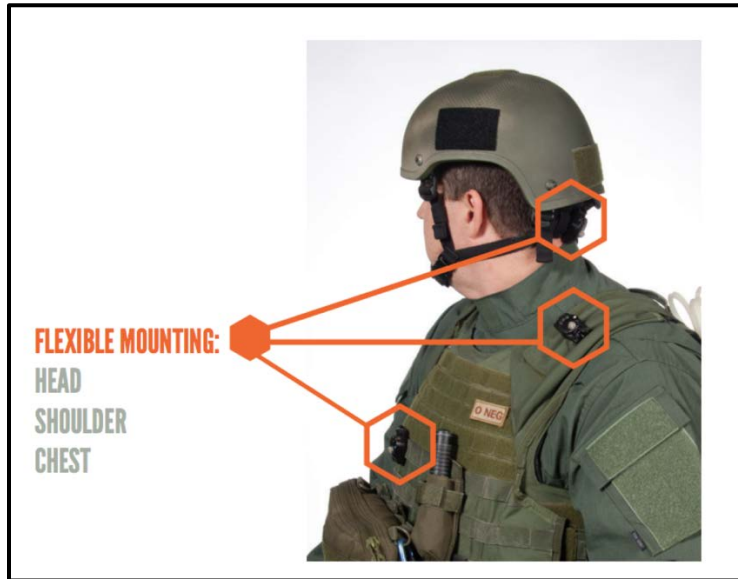
Figure 16. Blast Gauge placement on soldier: chest, shoulder, and head (nape pad). Source: The Blast Gauge System (n.d.).
