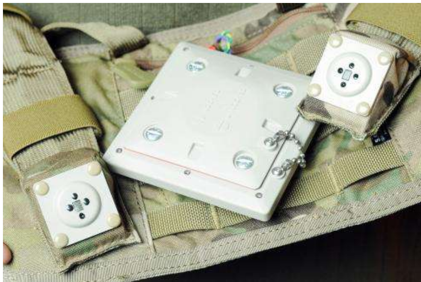
Figure 3. Components of I-BESS. Source: Becker (2013).
