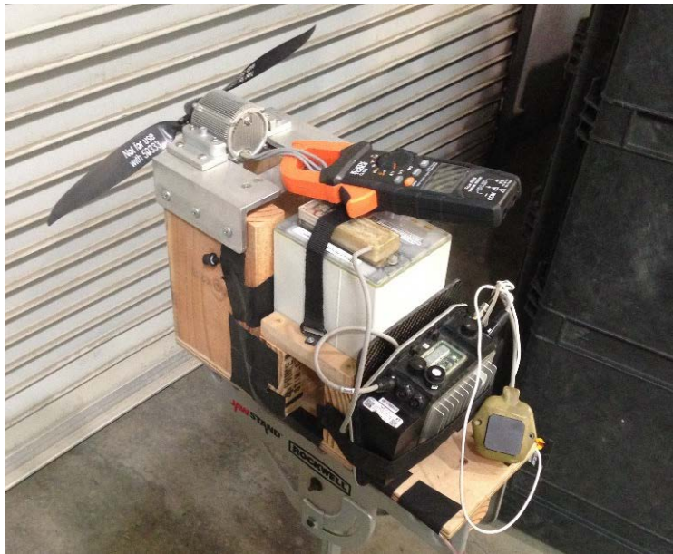
Figure 9. Motor test stand at ERI with digital clamp meter attached
