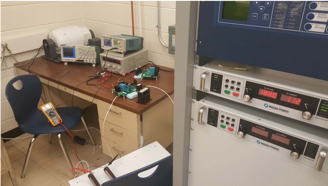
Fig 32. Hardware test of BoCBB in Boost mode
