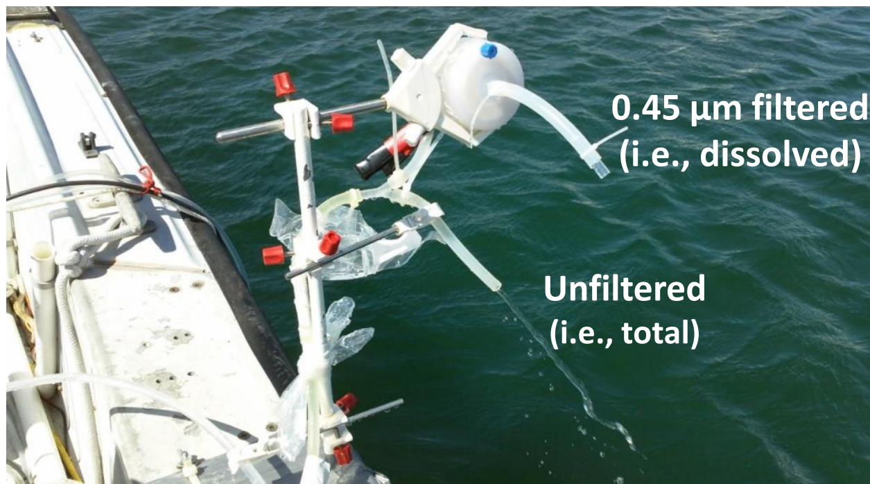
Figure 9. Peristaltic pump set up for collection of unfiltered and filtered water chemistry samples.
