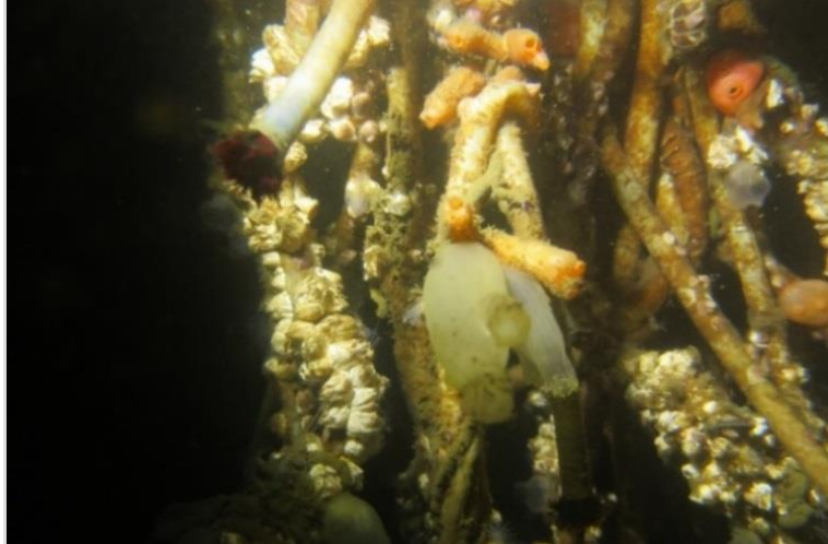
Figure 1. Example of biofouling density and diversity on the hull of the ex-INDEPENDENCE observed during pre-removal inspections.
