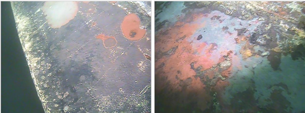
Figure 2. Top edge of port bilge keel showing paint (left) and top of port bilge keel showing paint and areas of bare hull (right).
