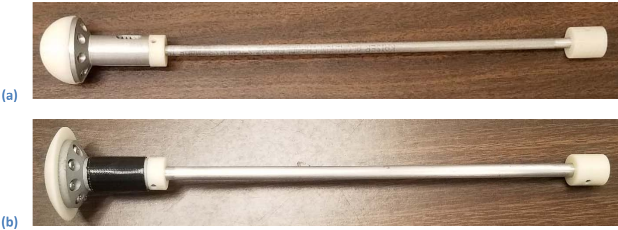
Figure 2-2. (a) The original projectile from PMHS testing (2017) and (b) the modified design to minimize penetration risks in animal testing.
