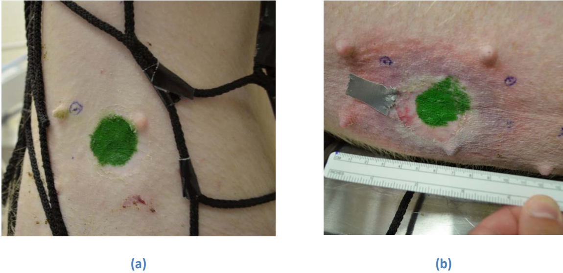
(a) (b) Figure 3-3. Comparison of tissue response to a stomach impact on a (a) cadaver specimen (69 m/s) and a (b) live anesthetized specimen (71 m/s). Green paint was used to paint the projectile and marks the exact impact site.
