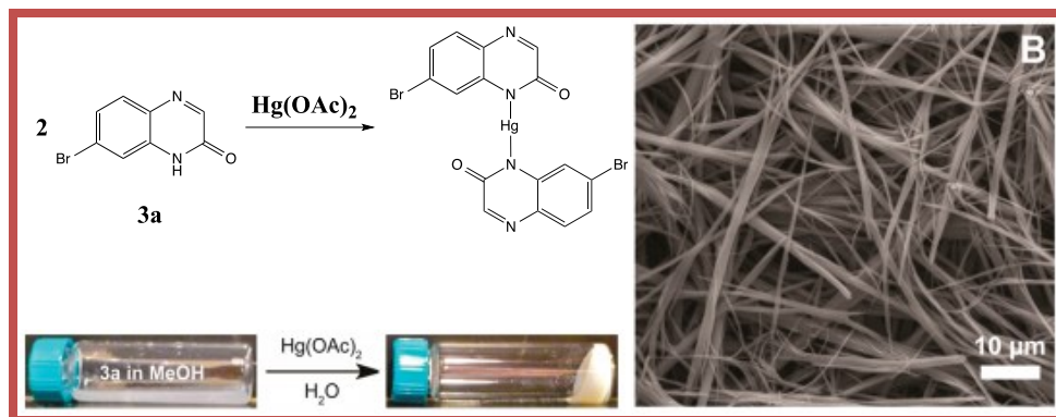
Figure 1.24: Reaction of quinoxalinone with mercury forms a hydrogel (Left). SEM of the hydrogel (Right). [88]
