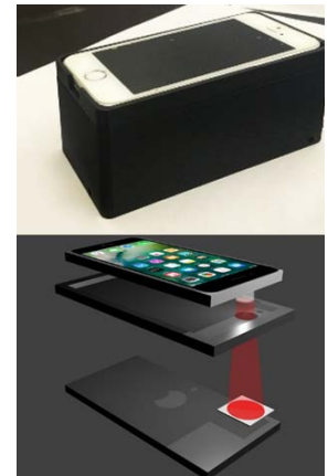
Figure 15. Photo (top) and schematic cut-away view (bottom) of porous silicon smartphone sensor with 3D printed box.
