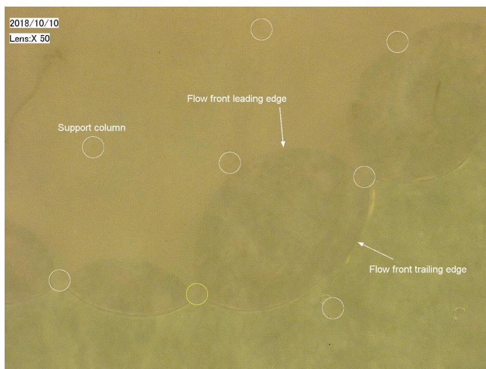
Figure 6: Micrograph illustrating the surface tension effect of sweat passing between reservoir support columns
