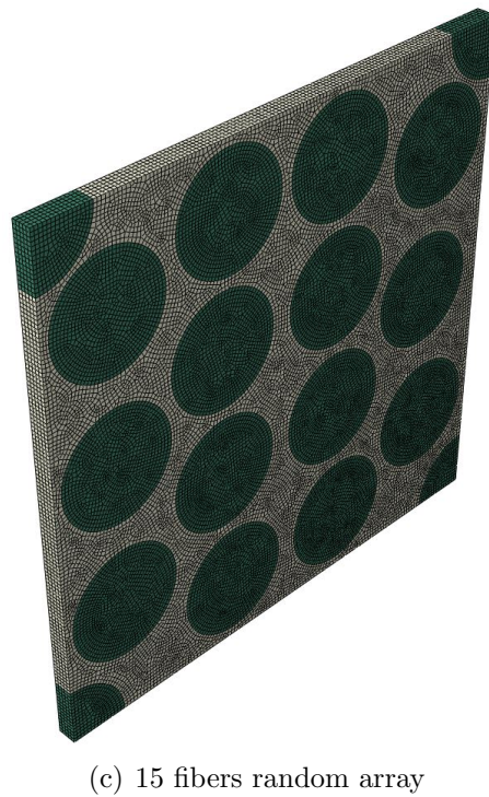
Figure 2.19: 3D RUC of UD composite (Fiber volume fraction=60%).
