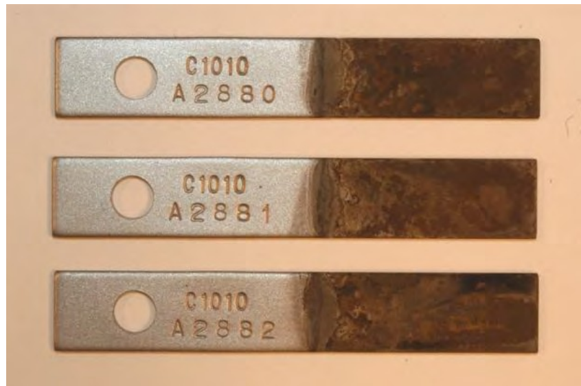
Figure 36. Macro photograph of the carbon steel coupon, after immersion testing in F-76 fuel/seawater mixture. The portion that was immersed in the F-76 fuel was on the left, and the portion immersed in the seawater was on the right. Some oxidation and general corrosion were also evident on the portion that was immersed in the seawater. Mag.: 1.2X
