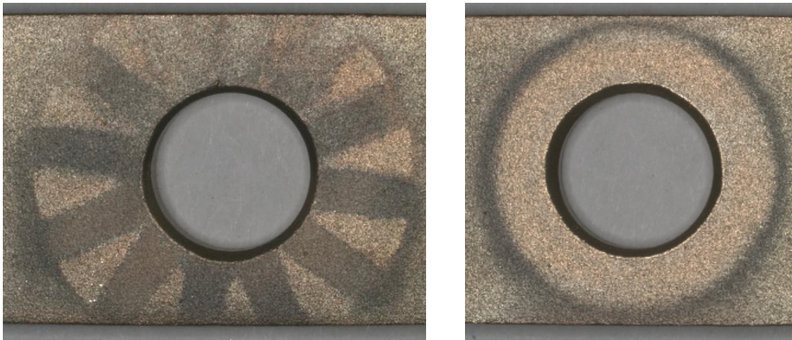
Figure 12. Macrophotograph of Cu-Ni alloy CDA 706, after immersion testing in the DSH fuel as a crevice corrosion assembly. Note the stains that developed at the crevice washer (left) and flat washer (right) sites. Mag.: 10X
