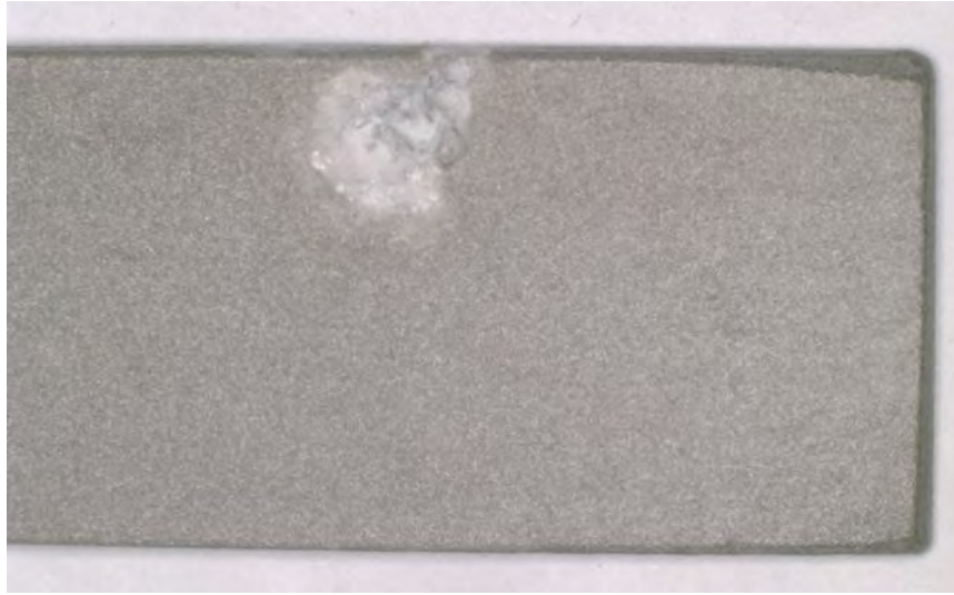
Figure 20. Stereophotograph of one (1) of the aluminum coupons, after immersion testing in the DSH fuel/seawater mixture. Note the pit present in the seawater side of the coupon. Mag.: 8X
