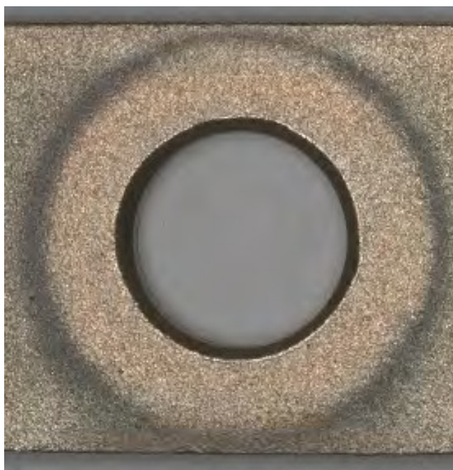
Figure 13. Opposite side of the coupon shown in Figure 12. Macro photograph of Cu-Ni alloy CDA 706, after immersion testing in DSH fuel as a crevice corrosion assembly. Note the stains that are evident on the flat washer side. Mag.: 10X
