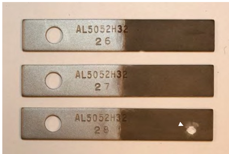
Figure 27. 35mm macrophotograph of the aluminum coupons, after immersion testing in F-76 fuel/seawater mixture. Note the pit present on the bottom coupon that was immersed in the seawater (identified by the white arrow). The portion that was immersed in the fuel was on the left, and the portion immersed in the seawater was on the right. Mag.: 0.5X
