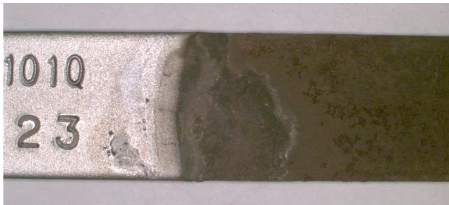
Figure 30. Macrophotograph of a carbon steel coupon, after immersion testing in the DSH fuel/sea water mixture. The portion that was immersed in the DSH fuel was on the left, and the portion immersed in the seawater was on the right. Oxidation, general corrosion, and pitting were evident at the fuel/sea water interface as well as on the portion that was immersed in the seawater. Mag.: 5X
