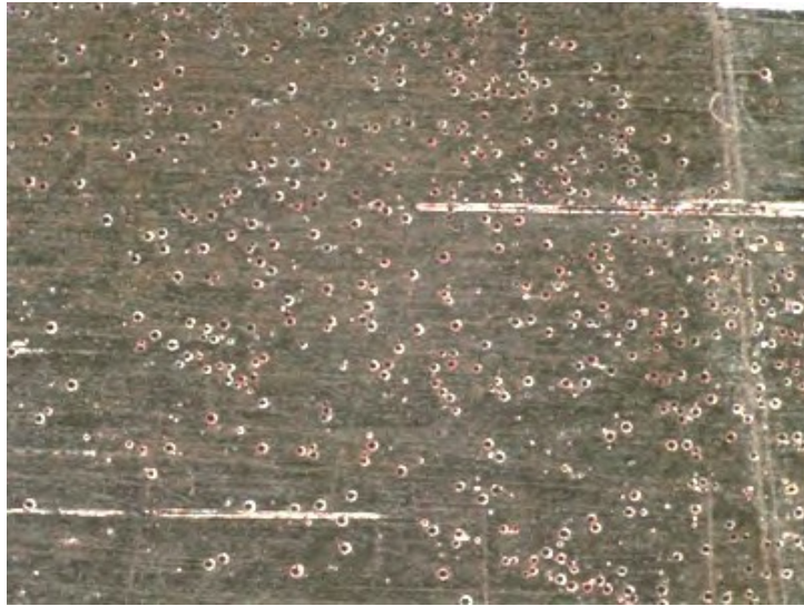
Figure 6. Macro photograph of a carbon steel coupon that had the electrodeposited zinc plating, static immersion tested in the F-76 fuel. Fine pits were observed. Mag.: 50X
