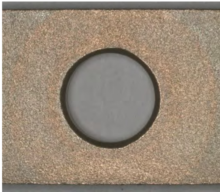
Figure 15. Opposite side of the coupon shown in Figure 14. Macrophotograph of Cu-Ni alloy CDA 706, after immersion testing in HDCD-1 fuel as a crevice corrosion assembly. There was evidence of staining on the flat washer side. Mag.: 10X
