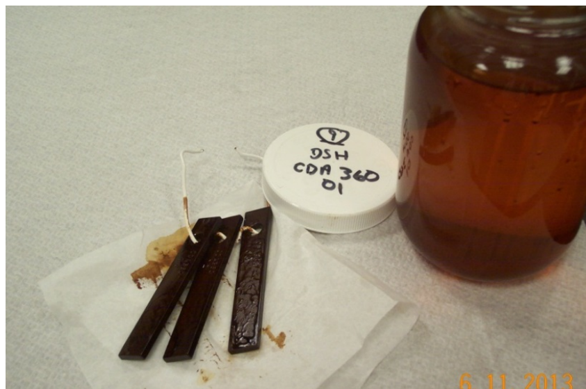
Figure 7. 360 leaded brass alloy exposed to DSH for 180 days at 120 °F became coated with a thick, black, tacky material.
