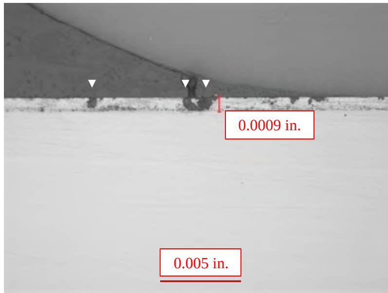
Figure 8. Photomicrograph of a carbon steel coupon that had the electrodeposited zinc plating, static immersion tested in the F-76 fuel. Fine pits, indicated by the white arrows, are evident in the zinc plating, extending to a maximum depth of 0.0009 in. As polished, Mag.: 200X
