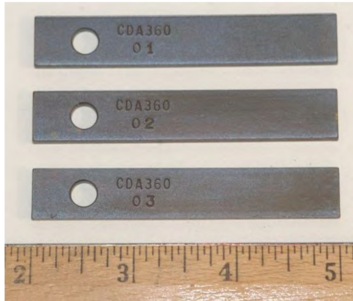
Figure 4. Macro photograph of the leaded brass coupon that were immersion tested in the DSH fuel. Note the dark blue colored appearance.
