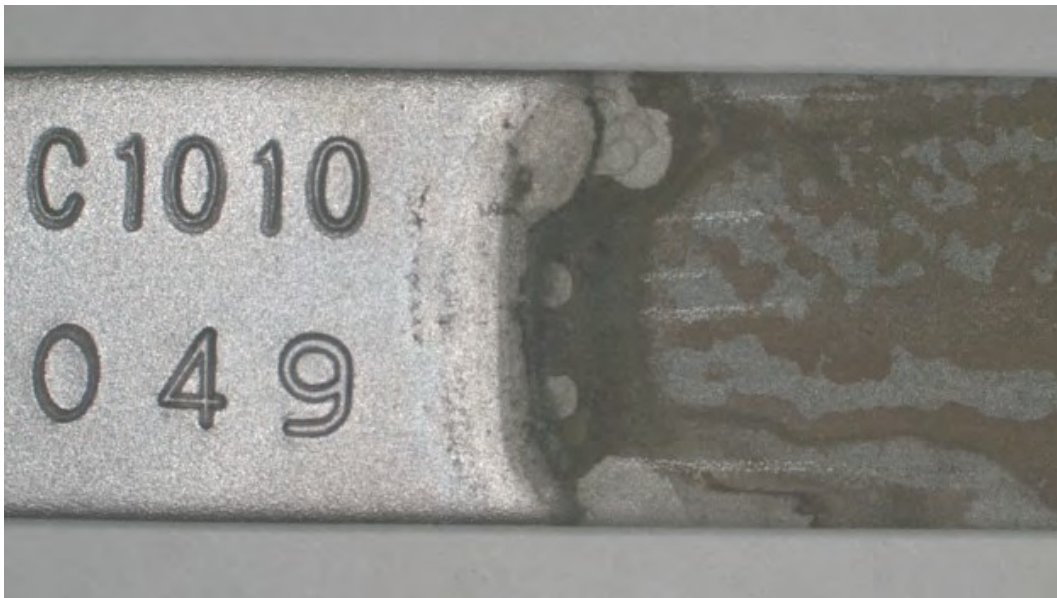
Figure 34. Macro photograph of a carbon steel coupon, after immersion testing in the HDCD-2 fuel/seawater mixture, showing an enlarged view of the fuel/seawater interface. The portion that was immersed in the HDCD-2 fuel was on the left, and the portion immersed in the seawater was on the right. Oxidation, general corrosion and pitting were evident, particularly at the fuel/seawater interface. Mag.: 10X
