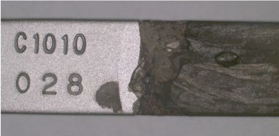
Figure 38. Macrophotograph of a carbon steel coupon, after immersion testing in the DSH fuel/deionized mixture. The portion that was immersed in the DSH fuel is on the left, and the portion immersed in the deionized water is on the right. Oxidation, general corrosion and pitting are evident on the deionized water side. The largest pitting was observed on the fuel side, directly adjacent to the fuel/deionized water interface. Mag.: 5X
