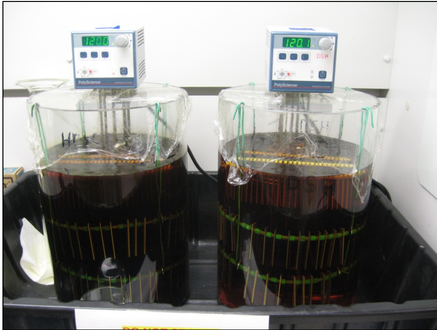
Figure 4. Laboratory set-up for flow test. Unit on tank is a combination circulator pump and heating element.
