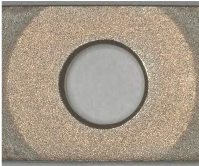
Figure 17. Opposite side of the coupon shown in Figure 16. Macro photograph of Cu-Ni alloy CDA 360, after immersion testing in HDCD-2 fuel as a crevice corrosion assembly. Note the stains that are evident on the flat washer side. Mag.: 10X
