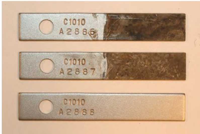
Figure 44. Macrophotograph of the carbon steel coupons, after immersion testing in the F-76 fuel/deionized water mixture. The portion that was immersed in the fuel was on the left, and the portion immersed in the deionized water was on the right. Oxidation and general corrosion were evident on the portion that was immersed in the deionized water on the top two (2) coupons. There was some attack noted in the water side in close proximity to the fuel/deionized water interface. The bottom coupon, for some unknown reason, was not corrosively attacked. SEM/EDS analysis verified that the coupon was carbon steel; the lack of oxidation on the deionized water side cannot be explained. Mag.: 0.5X
