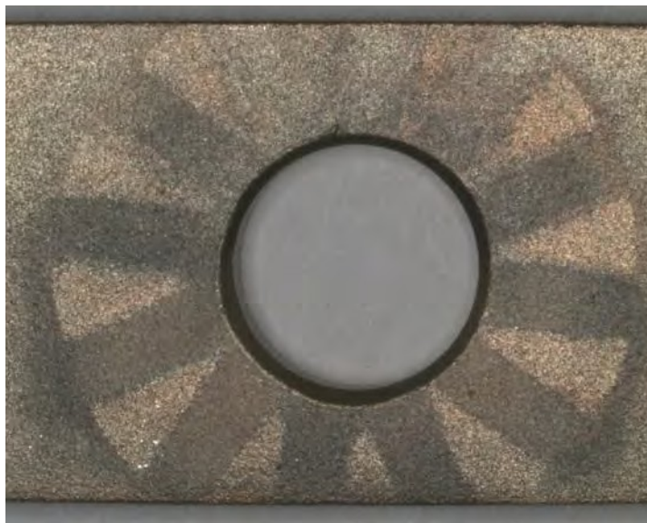
Figure 12. Macro photograph of Cu-Ni alloy CDA 706, after immersion testing in DSH fuel as a crevice corrosion assembly. Note the stains that developed at the crevice washer site. Mag.: 10X
