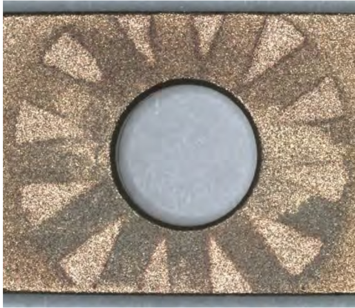
Figure 18. Macrophotograph of Cu-Ni alloy CDA 360, after immersion testing in F-76 fuel as a crevice corrosion assembly. Note the stains that developed at the crevice washer site. Mag.: 10X
