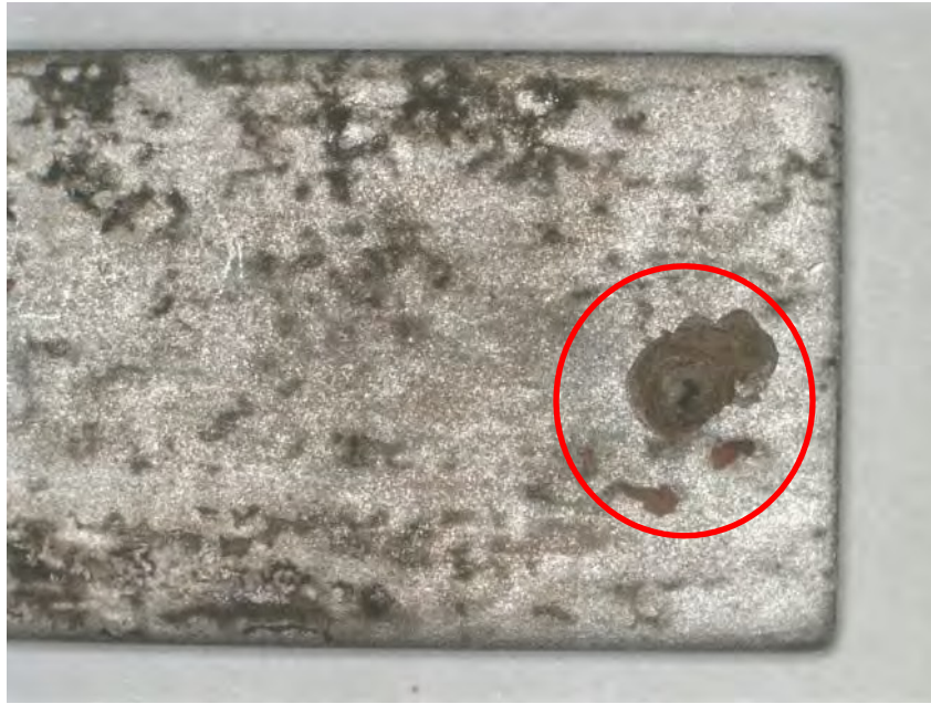
Figure 42. Macro photograph of a carbon steel coupon, after immersion testing in the HDCD-2 fuel/deionized water mixture which shows an enlarged view of one (1) of the coupons that was immersed in the deionized water portion. Oxidation, general corrosion and pitting were evident. A cluster of pits was identified within the red circle. Mag.: 10X
