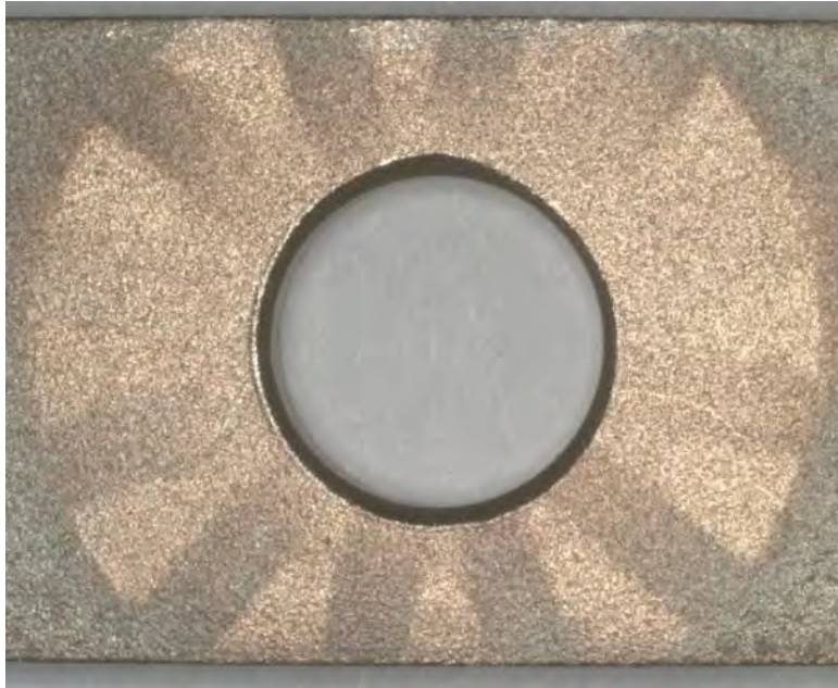
Figure 16. Macro photograph of Cu-Ni alloy CDA 360, after immersion testing in HDCD-2 fuel as a crevice corrosion assembly. Note the stains that developed at the crevice washer site. Mag.: 10X
