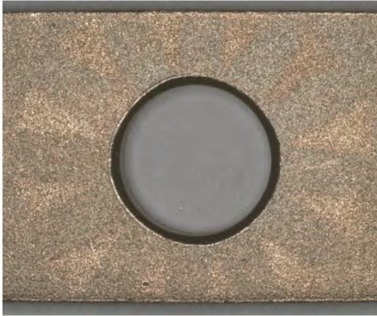
Figure 14. Macrophotograph of Cu-Ni alloy CDA 706, after immersion testing in HDCD-1 fuel as a crevice corrosion assembly. Note the stains that developed at the crevice washer site. Mag.: 10X
