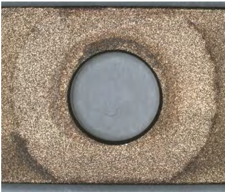
Figure 19. Opposite side of the coupon shown in Figure 18. Macrophotograph of Cu-Ni alloy CDA 360, after immersion testing in F-76 fuel as a crevice corrosion assembly. Note the stains imparted on the flat washer side. Mag.: 10X
