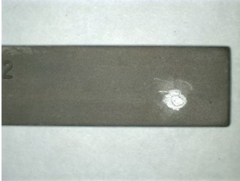
Figure 28. Enlarged view of the bottom coupon shown in Figure 27. The pit is located on the seawater side. Mag.: 4X
