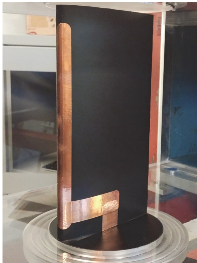
Figure 40. Model NACA 0015 Airfoil 6 inch chord 10 inch span Single DBD plasma actuator centered on the leading edge with 0.45 mm of PVC dielectric separation.
