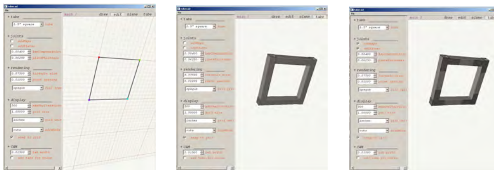
Figure 14: TubeCAD turns a sketch into tubes, with slot/tab connections and gussets optional
