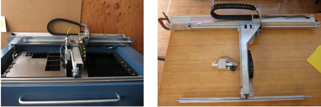
Figure 6: Two-axis cutter, installed (left) and alone (right)
