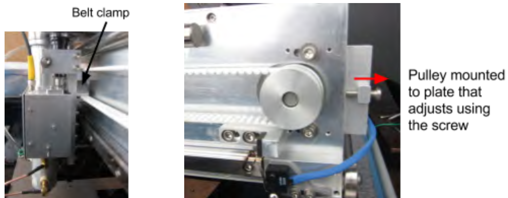
Figure 29: Example from the mechanics kit instructions relating concepts to the machine
