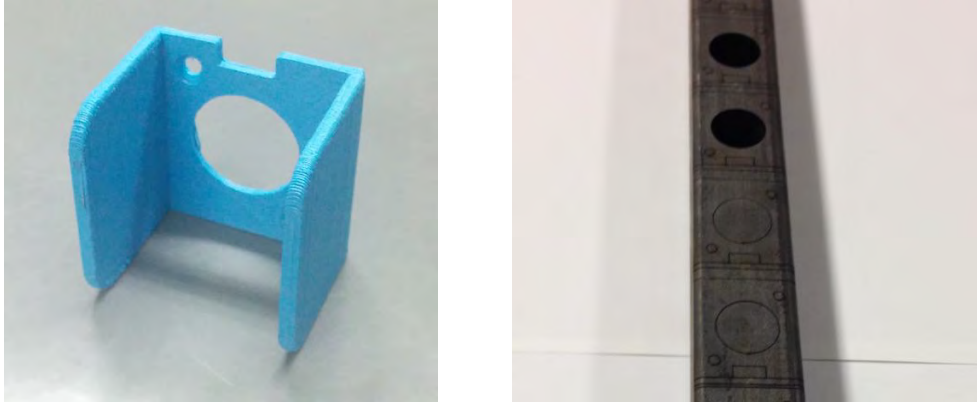
Figure 22: A switch cover 3D printed (left), now cut from square tube (right)
