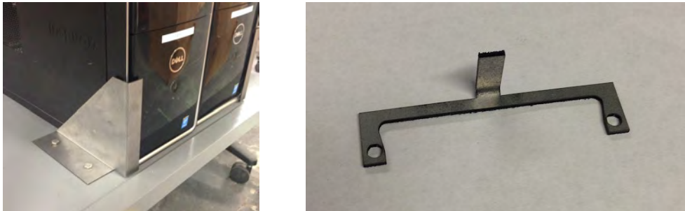
Figure 23: Two more brackets cut and bent at MARMC
