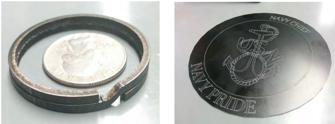
Figure 21: MARMC custom produced parts – split ring (left) and engraved plaque (right)
