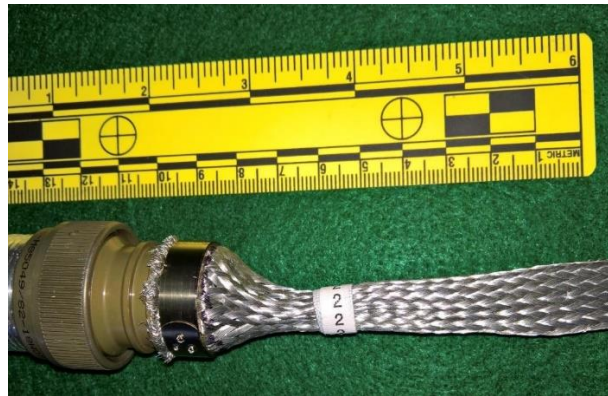
Figure 3: Optimized Spring Band Installed on a Typical EWIS Connector Accessory (M85049/82)
