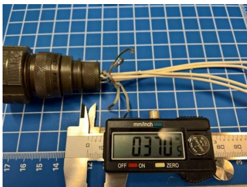
Figure 4: Typical Banding Platform Width Measured on an M85049 Accessory (N-dimension)
