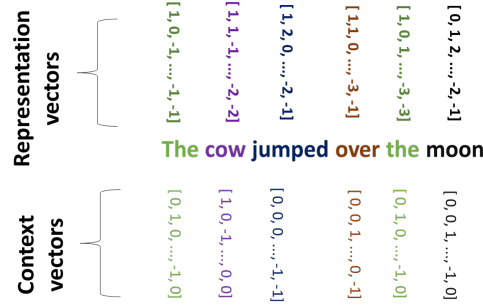
Figure 6: An example illustrating the naive Random Indexing algorithm with unigram atomic units and a (2, 2) -context window as context
