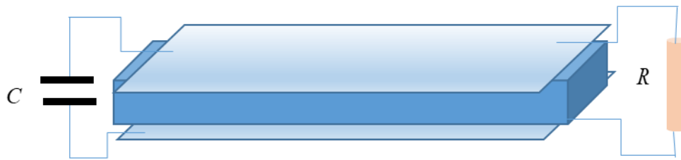
Fig. 2 Electric circuit with a pyroelectric charger (sandwich), capacitor, and resistor
