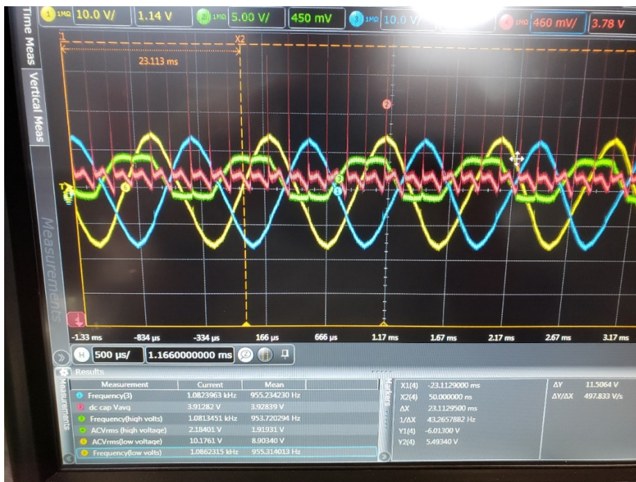
Figure 61. Breakdown in Rectifier Output
